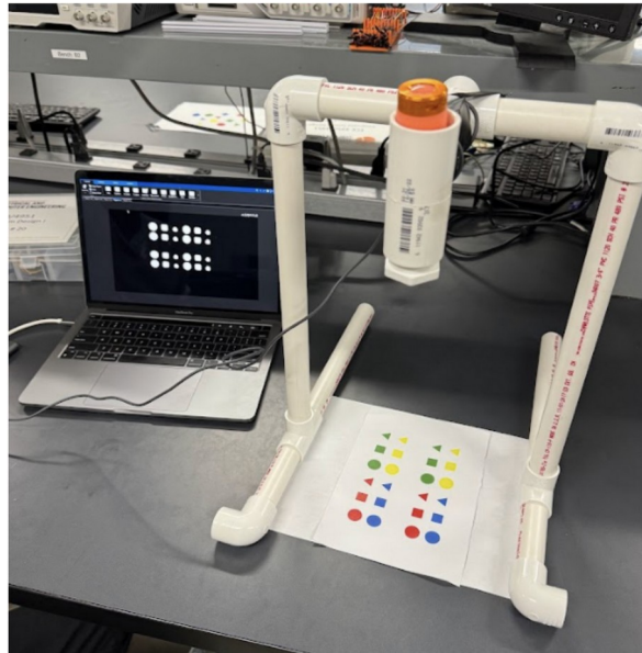
Figure 1: Camera System with PVC Rig
