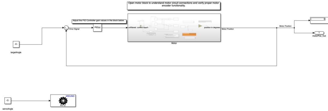
Figure 10. Simulink motor model for driving DC and servo motor
